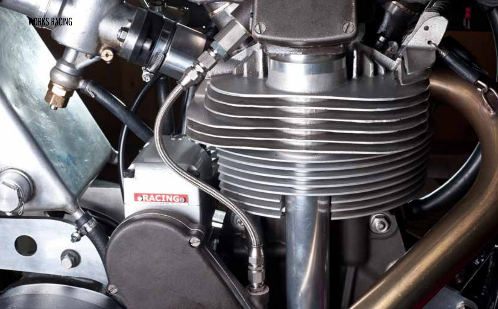
► Note Works Racing's own exhaust, the machined-from-solid barrel, updated Norton logo on the bevel cover and the utter absence of oil mess
